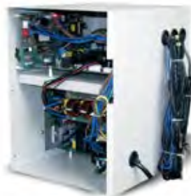
Inverter Controller for HP Water Heater
